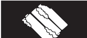
Remove dead batteries from equipment and all batteries from equipment you know you are not going to use for a long time. Otherwise the batteries may leak and cause damage.
