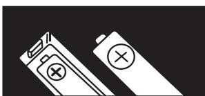
Take care to fit your batteries correctly, observing the plus and minus marks on the battery and appliance. Incorrect fitting can cause leakage or, in extreme cases, fire or even an explosion.
