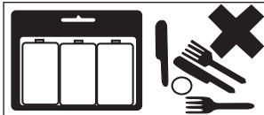
Store unused batteries in their packaging and away from metal objects which may cause a short-circuit resulting in leakage or, in extreme cases, fire or even an explosion.
