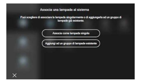
In the event of a pairing as an individual lamp, the procedure will be similar to the one used for the first lamp paired.
