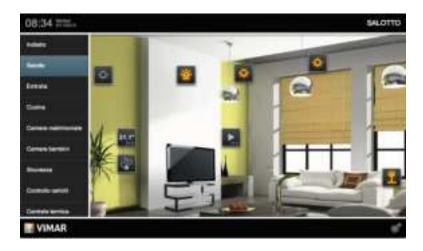
This way, you will be able to supervise a KNX system and manage other Vimar systems (By-alarm burglar alarm system, Elvox video door entry system and By-camera video surveillance) using a single touch screen.
