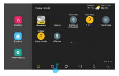
• In every screen, swipe up from the position shown (see subsequent figures) to display the device control panel (screen brightness, volume, etc.). Swipe up again to display further options only if the video door entry system is also present.
