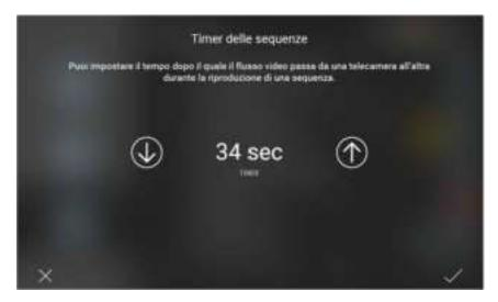
• Using and set the viewing time (minimum value 10 s, maximum value 60 s) and confirm with
