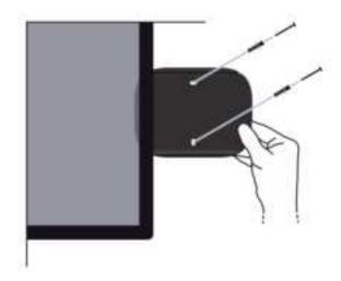
• Drill holes in the selected location for Wall Plugs. Insert Wall Plugs in the holes, and fix the Mounting Plate using the Screws (which can be found in the Accessory Kit).
