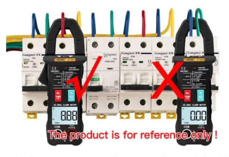
Before measurement, the measured current should be estimated and the appropriate range should be selected. When the current is not known, the maximum range should be selected and the range should be reduced appropriately according to the value. However, the range cannot be converted during measurement.
