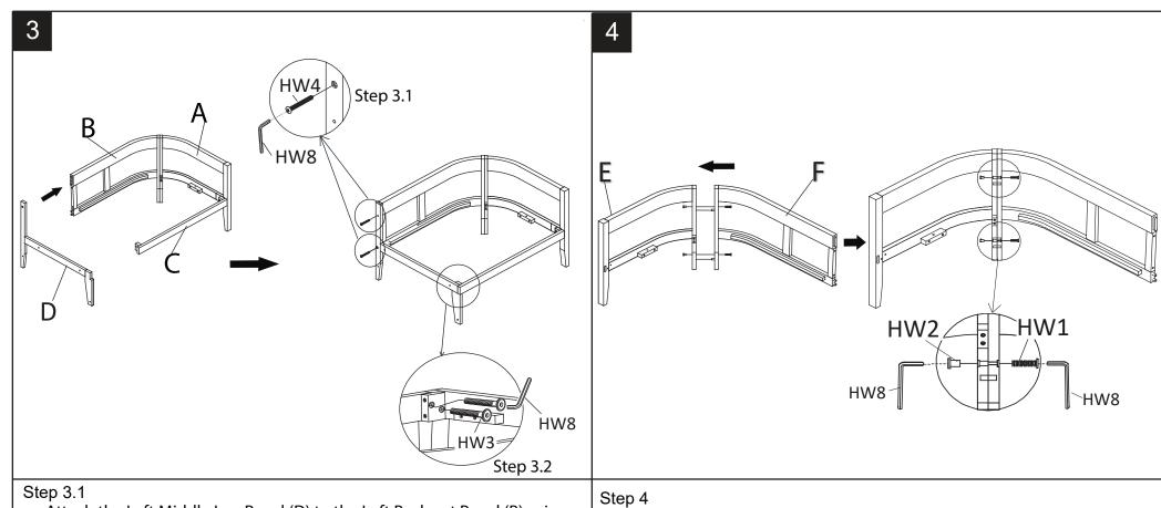
Attach the Left Middle Leg Panel (D) to the Left Backrest Panel (B) using Screws (HW4) and the Allen kay (HW8) as shown above.
