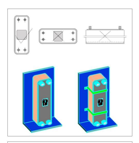
If the pipeline has vibration, longer pipe and higher thermal expansion, which will affect brazed plate heat exchanger. You'd better consider adopting the following devices: install rubber pad between brazed plate heat exchanger and bracket; compressor with shock absorber, and use corrugated pipe or other damping devices when straight pipe is longer.
