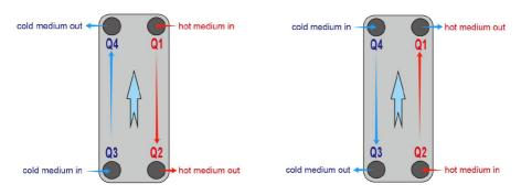
Note: When the PHE use to the evaporator, the refrigerant must  $Q2 \rightarrow Q1$  or  $Q3 \rightarrow Q4$ . When the PHE use to the condenser, the refrigerant must  $Q1 \rightarrow Q2$  or  $Q4 \rightarrow Q3$ . If you do not take over as shown in the figure above, there will be two media mixed together or no media outflow.
