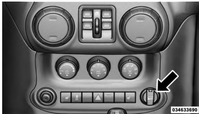
Front Power Outlet
