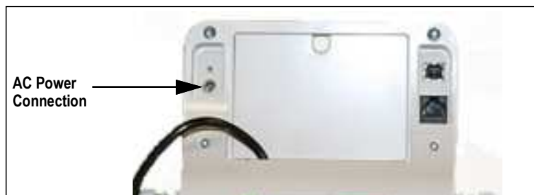
Figure 2-5. Power Connection Site
