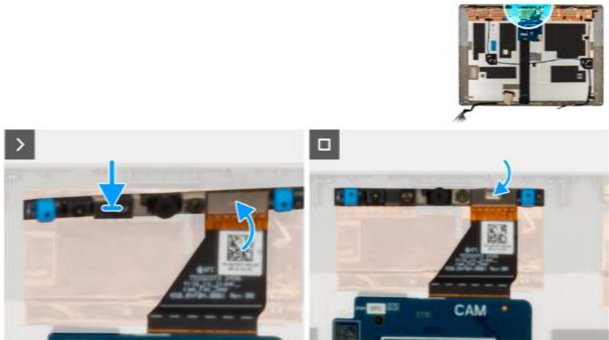
Figure 39. Installing the camera module display cable
