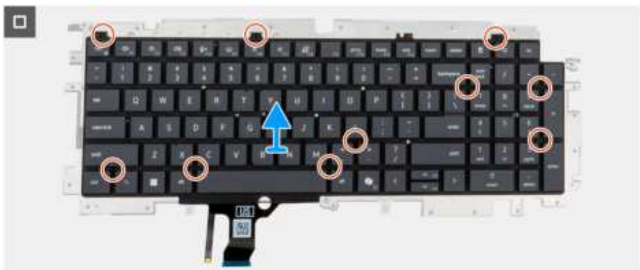
Figure 59. Removing the keyboard
