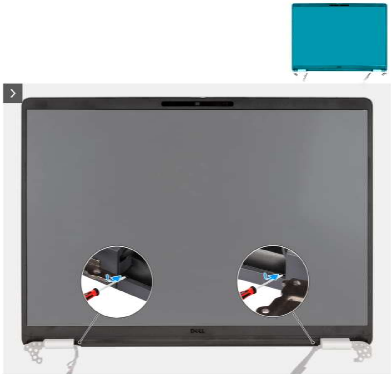
Figure 24. Prying the plastic bezel
