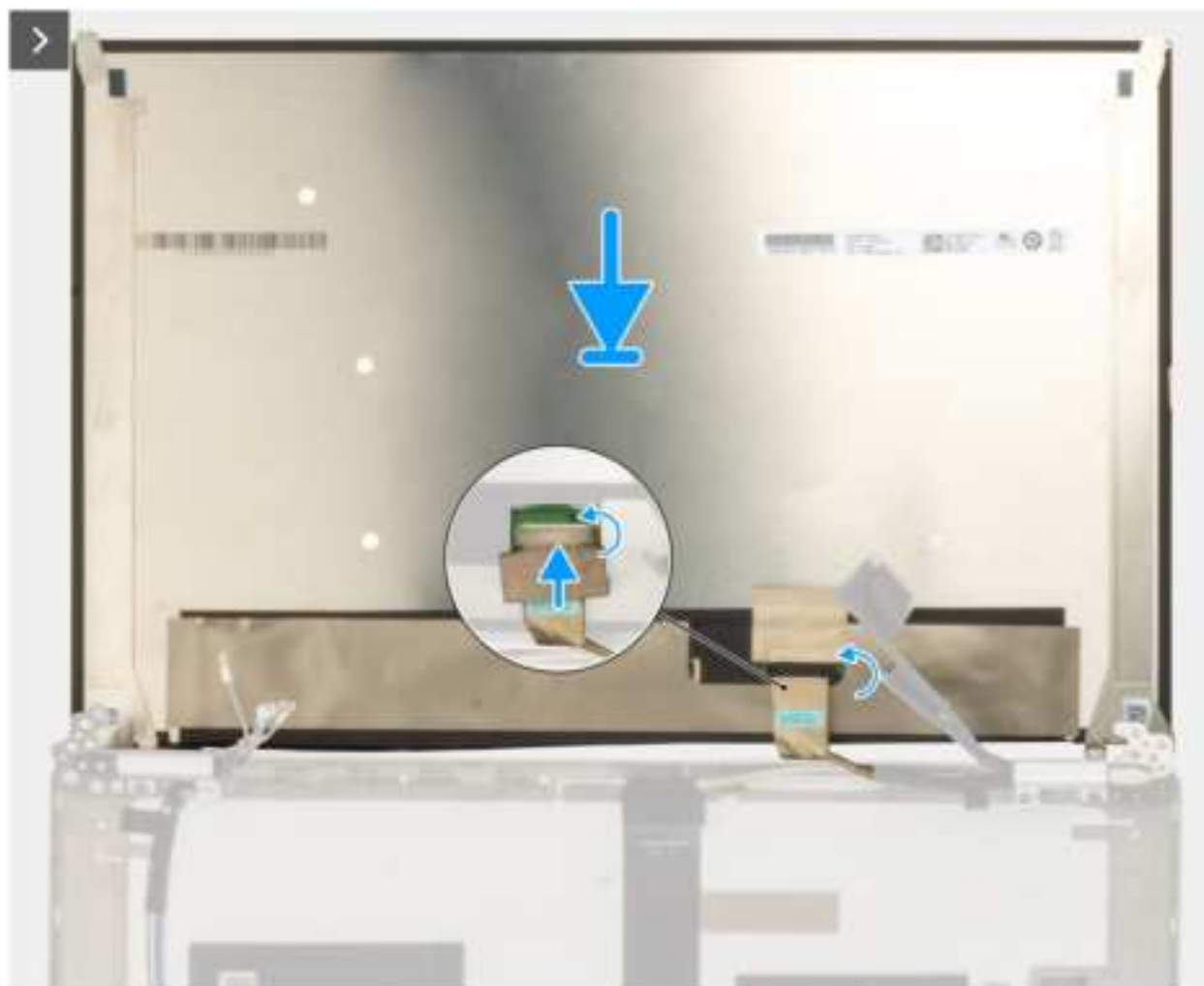
Figure 32. Installing the display panel
