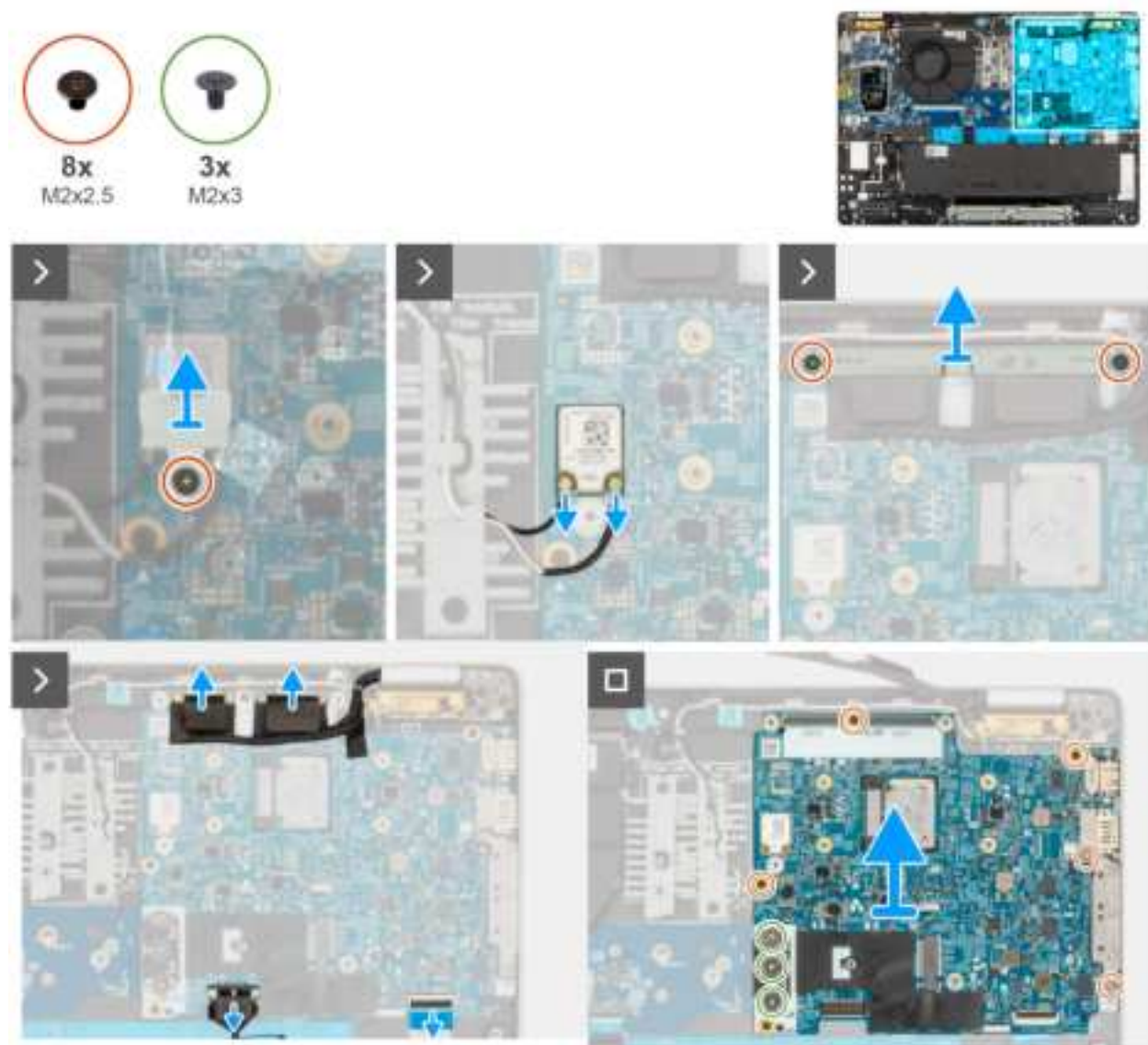
Figure 49. Removing the system board
