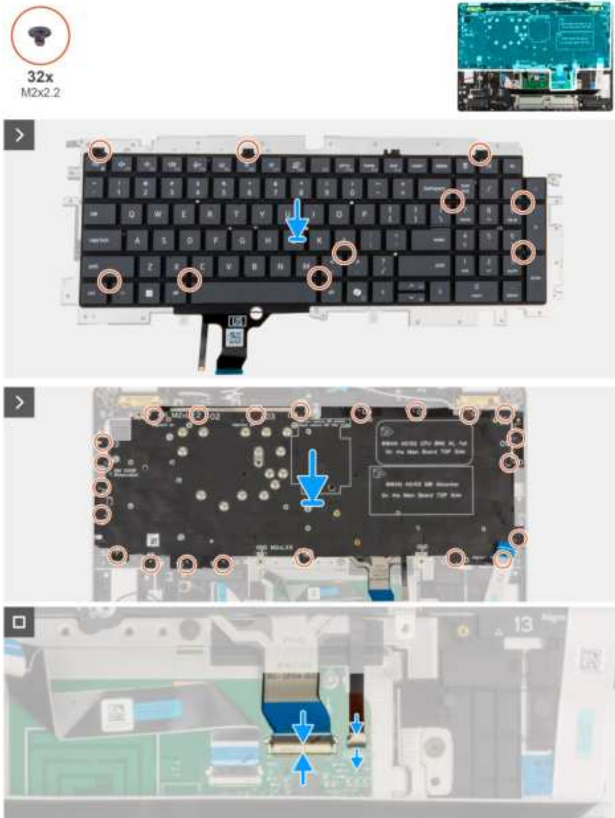
Figure 60. Installing the keyboard
