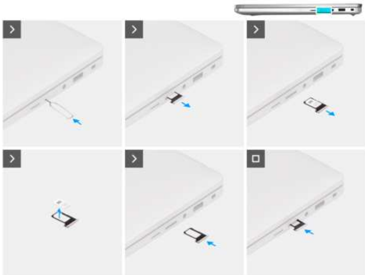
Figure 4. Removing the SIM card tray
