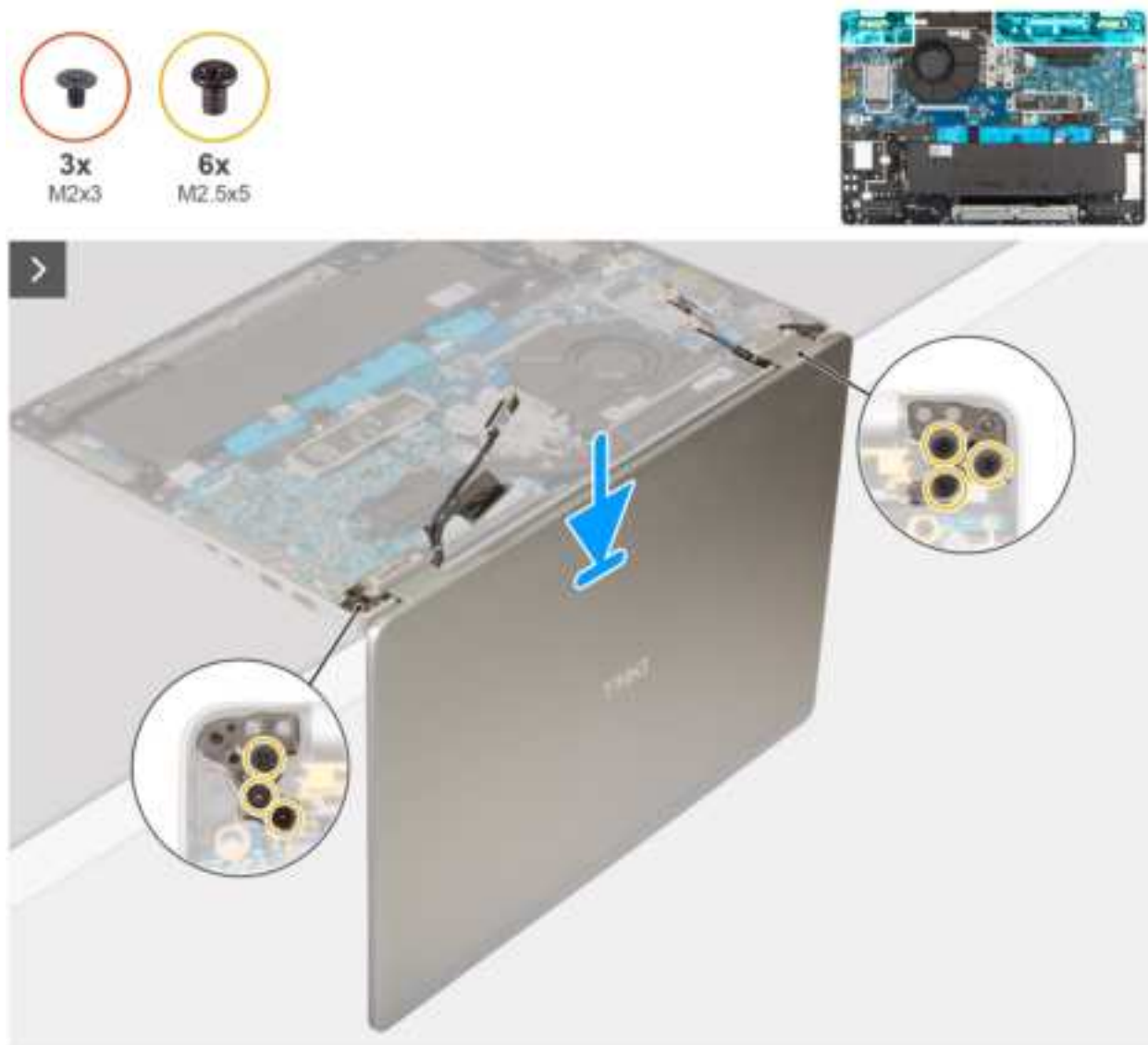
Figure 22. Installing the display assembly
