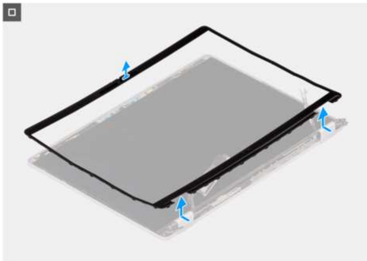
Figure 28. Removing the display bezel
