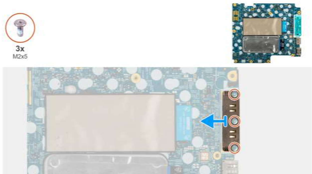
Figure 52. Removing the USB-C Connector Module
