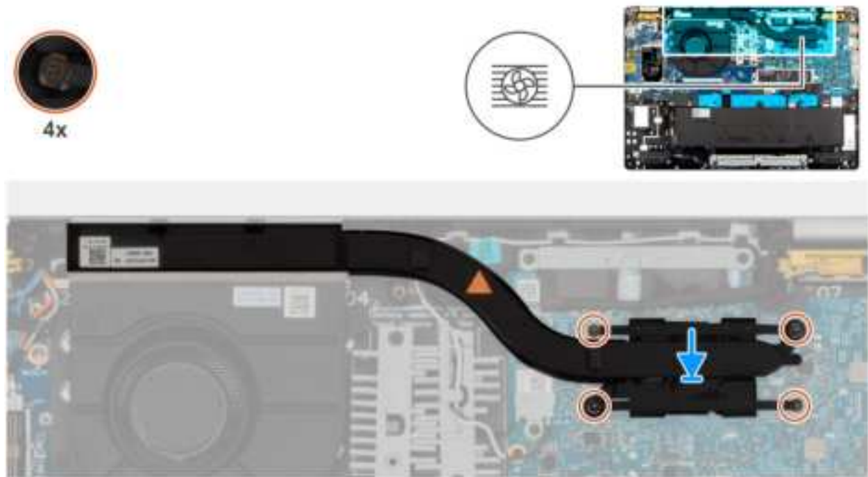
Figure 47. Installing the heat sink
