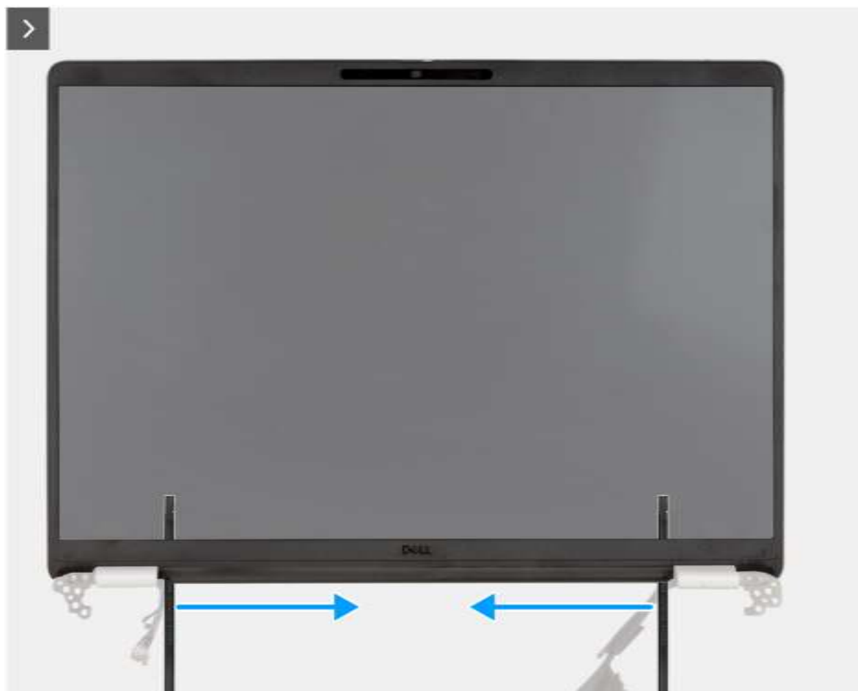
Figure 25. Prying the bezel along the sides
