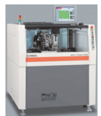
"Micro-prober" Conduction break inspection machine
