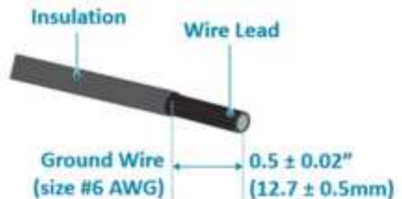
6-AWG green-and-yellow wire for grounding
