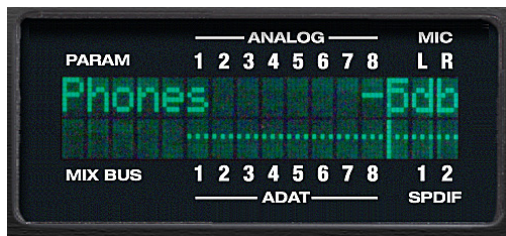
Figure 6-3: For many settings, the LCD “zooms in” on the setting as you adjust it.
