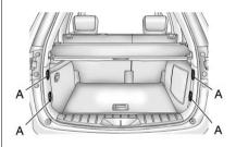
The vehicle may be equipped with four cargo tie downs (A) located in the rear compartment.
