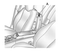
For vehicles with a center console storage, use the lever (A) on the front to open.
