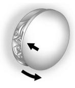
The tethered fuel cap is behind the fuel door on the vehicle's passenger side. To open the fuel door, push the rearward center edge in and release and the door will open. Turn the fuel cap counterclockwise to remove. Do not release the cap too soon or it will spring back. Reinstall the cap by turning it clockwise until it clicks.
