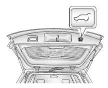
Press and release on the liftgate adjacent to the latch to close the liftgate.
