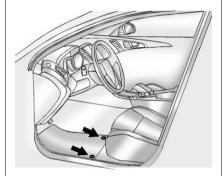
The driver side floor mat is held in place by two retainers.
