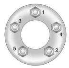
Tighten the wheel nuts firmly in a crisscross sequence, as shown.
