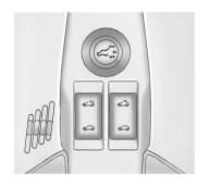
On vehicles with a power liftgate, the vehicle must be in P (Park) to use the power feature. The taillamps flash when the power liftgate moves.
