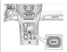
Press the "eco" (economy) button by the shift lever to turn this feature on or off. The "eco" light in the instrument cluster will come on when engaged. See Fuel Economy Light on page 5-22. A Driver Information Center (DIC) message "ECO MODE ON" is also displayed. See *Fuel System Messages on page 5-30* for more information.
