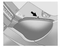
Locate the vertical headlamp aiming screws, which are under the hood near each headlamp assembly.  Turn the vertical aiming screw until the headlamp beam is aimed to the horizontal tape line. Turn it clockwise or counterclockwise to raise or lower the angle of the beam.
