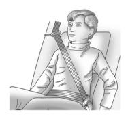
4. Buckle, position, and release the safety belt as described previously in this section. Make sure the shoulder portion of the belt is on the shoulder and not falling off of it. The belt should be close to, but not contacting, the neck
