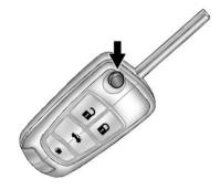
Press this button to extend the key. The key can be used for the ignition and all locks.
