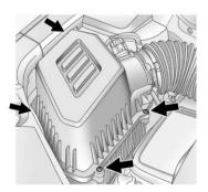
3. Remove the four air cleaner housing cover screws.
