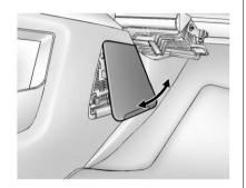
The instrument panel fuse block is located on the passenger side panel of the center console. To access the fuses, open the fuse panel door from the passenger side by pulling it out.
