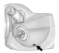
Vehicles with an automatic transmission are equipped with an electronic key lock release system.
