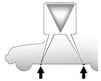
4. Position the jack lift head at the jack location nearest the flat tire. The location is indicated by a mark on the bottom edge of the front and rear door plastic molding. The jack must not be used in any other position.
