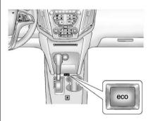
Press the "eco" (economy) button by the shift lever to turn this feature on or off. The "eco" light in the instrument cluster will come on when engaged, and a Driver Information Center (DIC) message "ECO MODE ON" displays. See Fuel Economy Mode on page 9-31.
