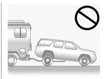
Notice: Towing the vehicle from the rear could damage it. Also, repairs would not be covered by the vehicle warranty. Never have the vehicle towed from the rear.
