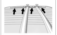
The roof rack cross rails can be locked in four positions along the roof rack side rails. These are the only positions that the cross rails will lock.
