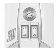
Choose the power liftgate mode by turning the dial on the switch until the indicator lines up with the desired position. The vehicle must be in P (Park).
