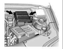
To remove the fuse block cover, squeeze the clips on the cover and lift it straight up. See Engine Compartment Overview on page 10-6.
