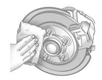
Remove any rust or dirt from the wheel bolts, mounting surfaces, and spare wheel. 12. Place the compact spare tire on the wheel-mounting surface.
