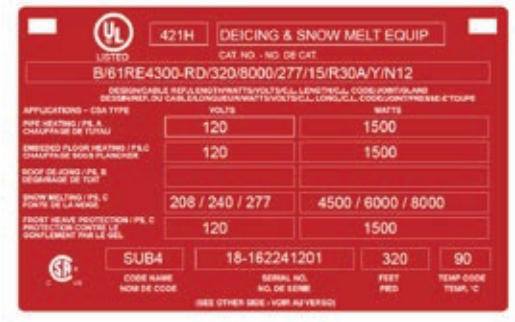
Figure 3: Typical SUA/SUB MI heating cable identification tag (front)
