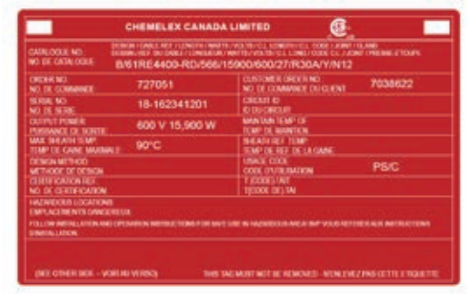
Figure 4: Typical heating cable identification tag for FFHP, HLR, FH and FFHPC cables (front)
