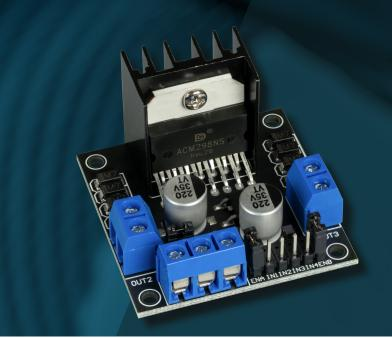
The MotoDriver 2 is a powerful and versatile expansion board for controlling and powering up to two DC motors. Equipped with the proven L298N H-bridge driver, the module enables precise control of motors in both directions of rotation and is ideal for applications in the fields of robotics, automation technology, model making or education.
