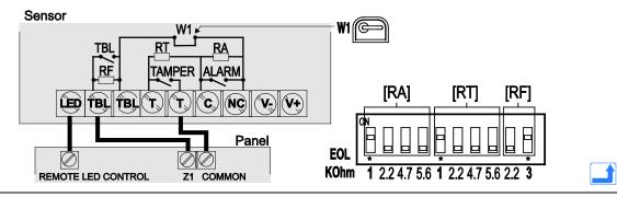
Alarm, Tamper and Trouble/Anti-Mask configured to two loops.
