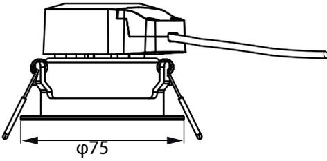
Cut-out hole diameter -  $\varnothing 68$ mm
