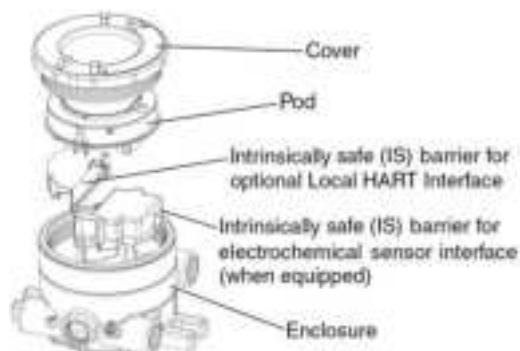
Figure 2. XNX exploded view
