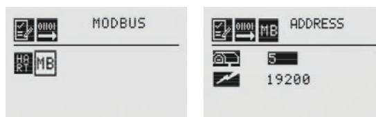
Figure 182. Modbus Configuration Display screen
