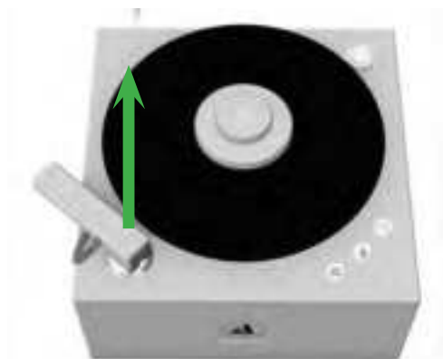
Pic. 7: Removing the cleaning- / suction arm
