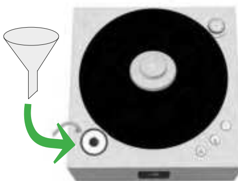
Pic. 8: Insert the filling funnel
