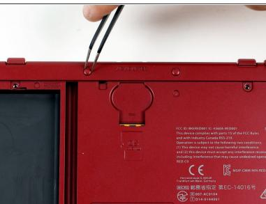
Using tweezers, carefully pop out the rubber bumpers located at the top side of the 3DS. Removing them will reveal another two 6mm screws. Remove these screws using a JIS #000 as well.
