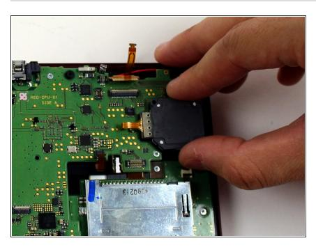
Lift the circle pad casing upward to remove it. There will be some friction, but it should not require excessive force.
