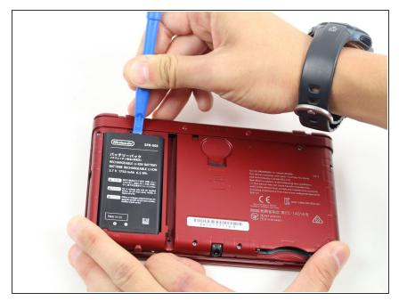
The battery is located on the left hand side of the 3DS - to remove, use the small gap located at the topmiddle and pull up with a pointed tool.
