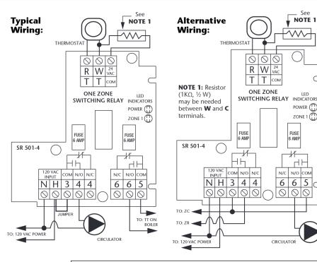
**NOTE 2:** When using Alternative Wiring diagram, the boiler operating control's ZC terminal will see the load of the circulator(s).
