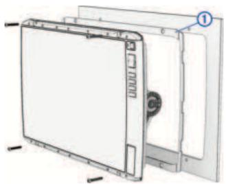
**12** Connect all necessary cables(*Connector View*, page 2), and turn the locking rings clockwise to secure the cables to device before placing it into the cutout.
