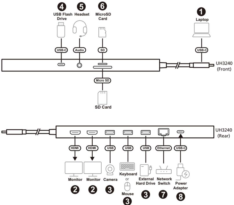
1. Connect a USB-C source device to the unit's USB-C host connector.
