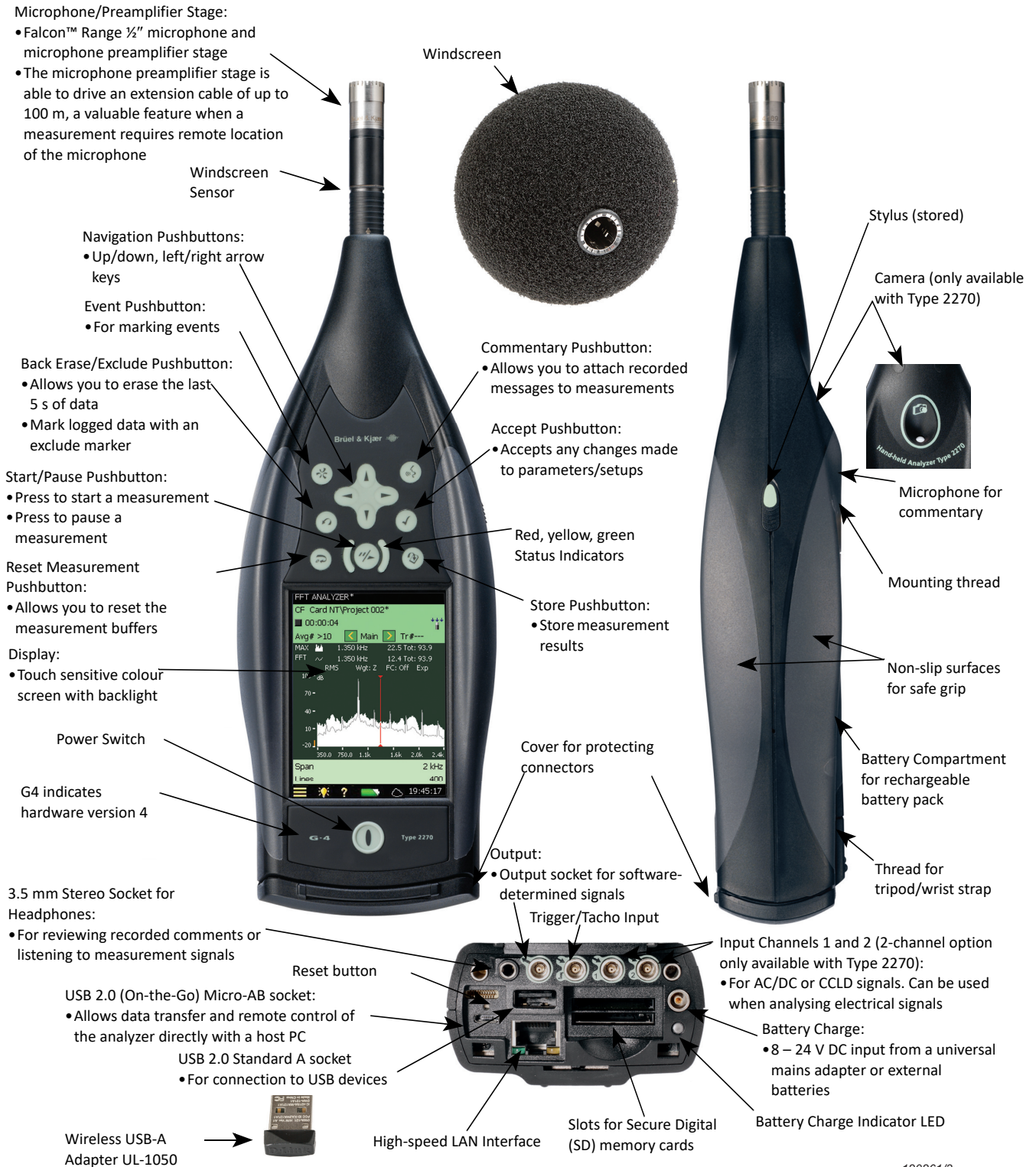
Fig. 1 Key features of Hand-held Analyzer Types 2250 and 2270
