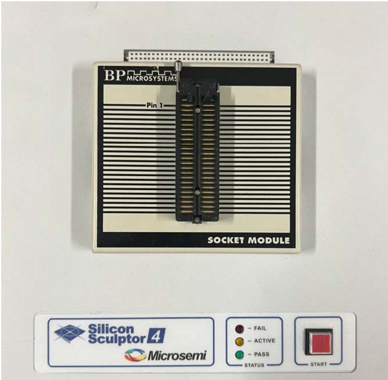
Figure 2. SM48D/SM48DB Socket Module Placed on SS4 Programmer
