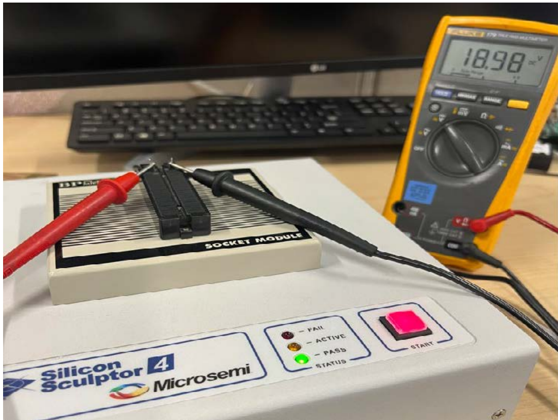
Figure 7. Voltage Measurement of the Pin 1
