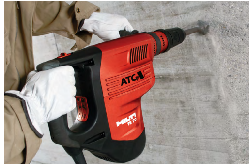
b) Surface roughening using brushing tool
