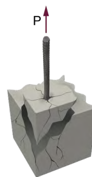
Fig. 2.11: Concrete cone breakout failure
