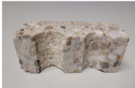
b) Difference between roughened & smooth borehole in concrete
