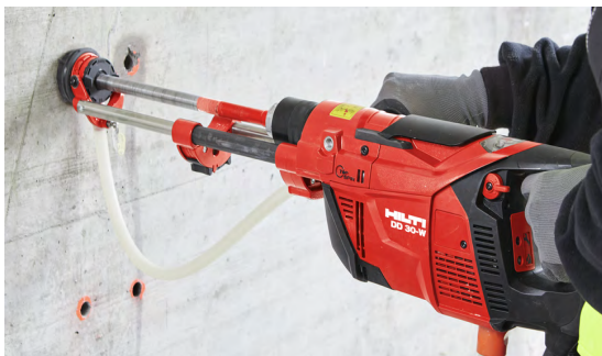
a) Diamond core drilling (Hilti DD 30-W)
