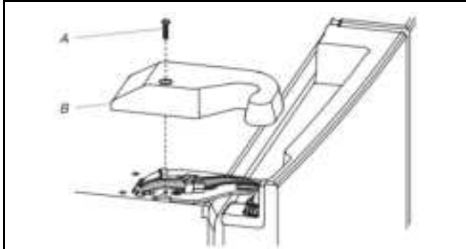
A. Top hinge cover screw
