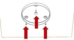
Offer up the base up to the ceiling and drill a suitable cable entry hole in the centre behind the base. The hole should be approximately 20mm in diameter.
