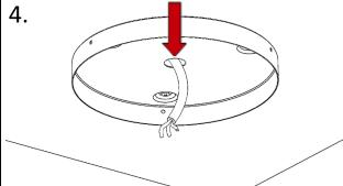
Feed the mains cable in through the drilled hole in the ceiling and through the base. Wire into the relevant terminals in the main housing and ensure the cable clamp is secured.
