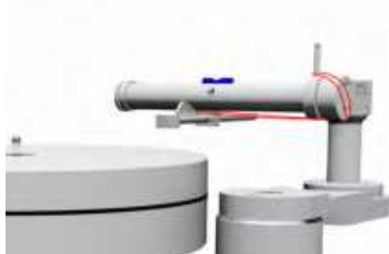
Pic. 8: Mounting the tonearm
