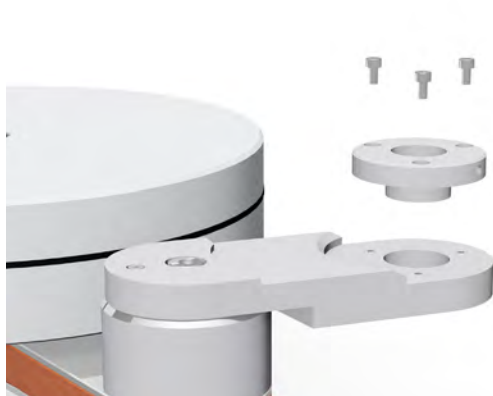
Pic. 5: Mounting the clamping ring
