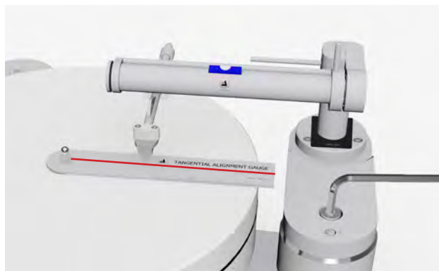
Pic. 21: Adjustment of the linear tracking
