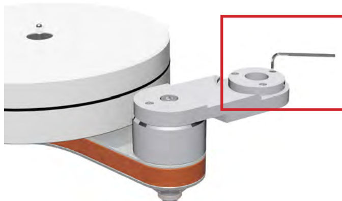
Pic. 6: Fixing the clamping ring
