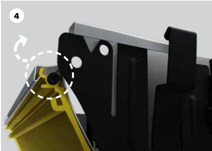
Pry open reflector edge from casing using a spudger tool
