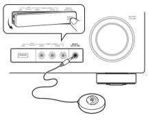
If you have a tripod, use it to place the microphone so that it's about ear level at your normal listening position. If you do not have a tripod, use some other object to install the microphone.<sup>1</sup>
