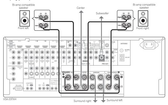
Bi-amping is when you connect the high frequency driver and low frequency driver of your speakers to different amplifiers for better crossover performance. Your speakers must be bi-ampable to do this (having separate terminals for high and low) and the sound improvement will depend on the kind of speakers you're using.
