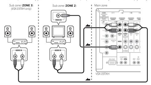
Different sources can be playing in two (VSX-21TXH)/three (VSX-23TXH) zones at the same time or, depending on your needs, the same source can also be used. The main and sub zone(s) have independent power (the main zone power can be off while one (or both) of the sub zone(s) is on) and the sub zone(s) can be controlled by the remote or front panel controls. However, you may need to specify the volume settings in ZONE Audio Setup on page 95.
