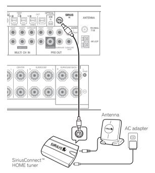
You will also need to connect the antenna and AC adapter to the SiriusConnect™ tuner.
