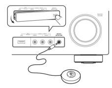
If you have a tripod, use it to place the microphone so that it's about ear level at your normal listening position. If you do not have a tripod, use some other object to install the microphone. 1
