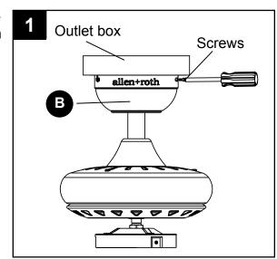
2. Remove the fan from the hook on the mounting bracket (A). Align the locking slots of the canopy (B) with the two screws in the mounting bracket (A). Push up to engage the slots, then turn clockwise to lock in place. Immediately tighten the two screws firmly.
