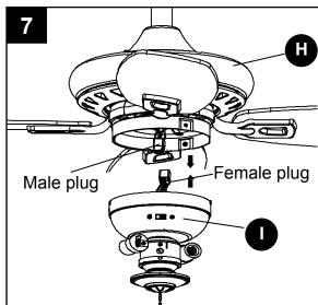
8. Attach the switch housing (I) to the switch housing cover on motor housing assembly (H). Align holes in switch housing (I) with holes on outer edge of the switch housing cover. Install the previously removed screws (Step 6, page 13) and tighten securely.
