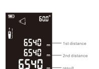
Add: short press ½ Subtract: long press ½ Measure the 1st distance, then press 🔽 add/subtract icon will appear on display, then press to measure the 2nd distance, the 2nd value will be automatically added to/ subtracted to the 1st value. Note: This process can be repeated as required.
