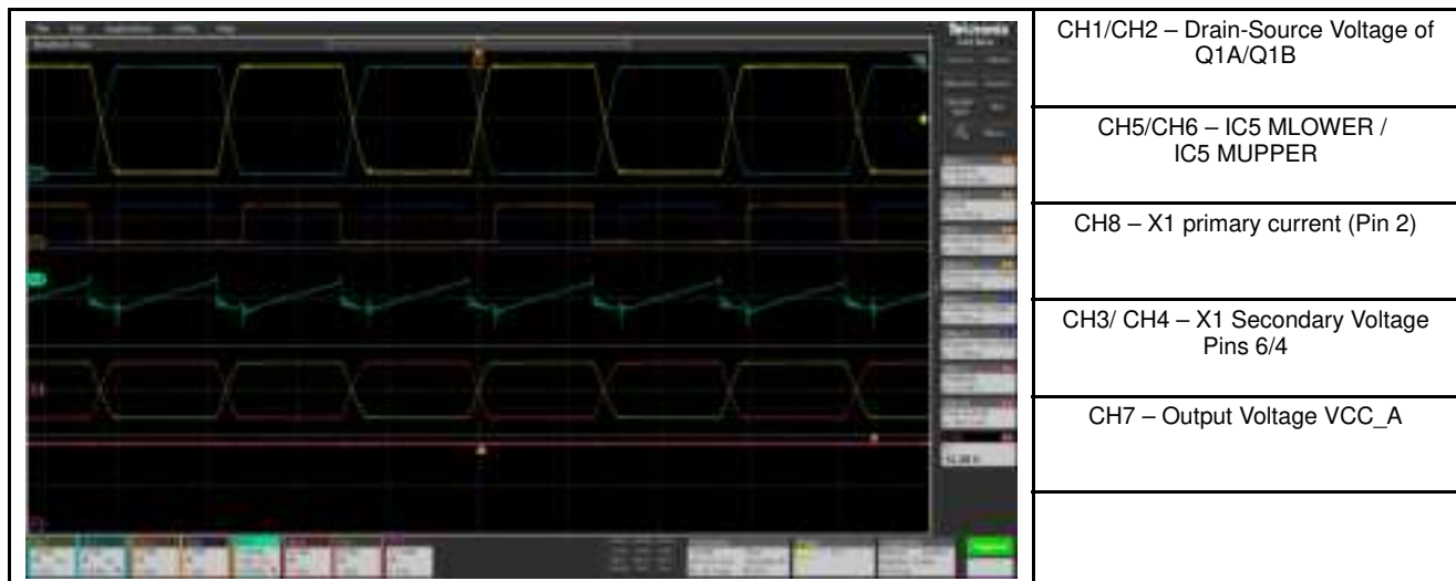
Figure 10. DC-DC Converter Waveforms Using R13 = 4.7 kΩ. Operating Frequency 358 kHz
