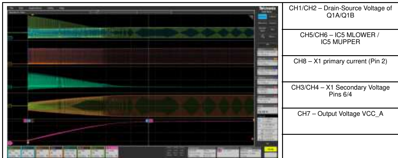
Figure 11. DC-DC Converter Start-up Sequence Waveforms
