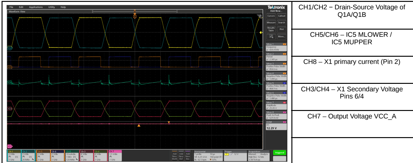
Figure 9. DC-DC Converter Waveforms Using R13 = 3.9 kΩ. Operating Frequency 426 kHz
