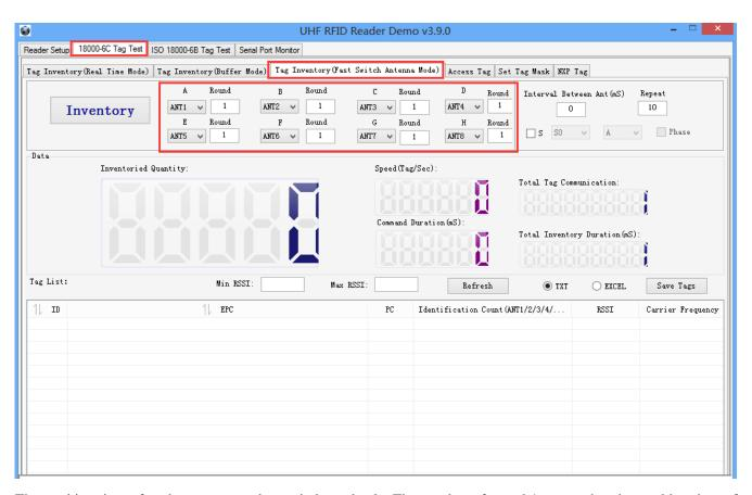
The working time of each antenna can be set independently. The number of round 1 means that the working time of the antenna is 50ms, and the number of round\*50ms is the working time of the antenna. Set the appropriate number of round according to the number of tags in front of the antenna. The default number of round is 1.
