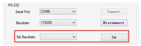
After the setting is successful, the new baud rate will be saved in the FLASH inside the reader, and will not be lost after the reader power off, restart the reader to make the setting effective. At this time, it must communicate with the reader at the new baud rate.
