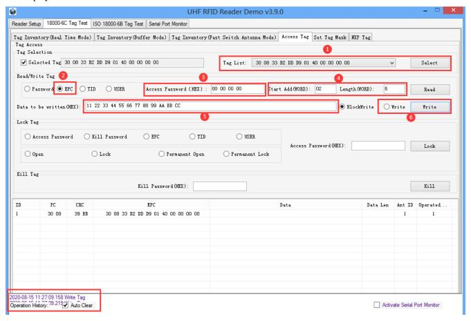
How many tags are successfully operated, how many pieces of data will be displayed in the list. Unlike reading tags, there is no content in the data column in the figure above. The user can read the same area of the tag again to verify that the data is written correctly. As shown below:
