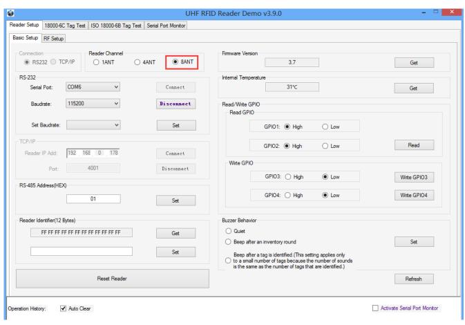
If the reader is connected via RS232, please select "RS232" in the connection mode, select the corresponding serial port number, and select the corresponding baud rate. The default baud rate is 115200. As shown below:
