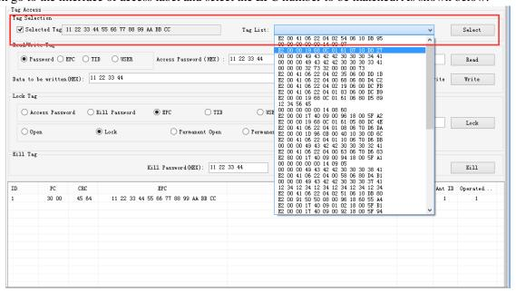
After the selection is completed, click the "Select" button, and the following figure will be shown after successful operation:
