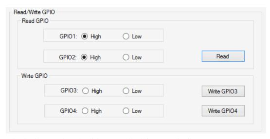
Users can read and write GPIO through serial commands in their own applications.
