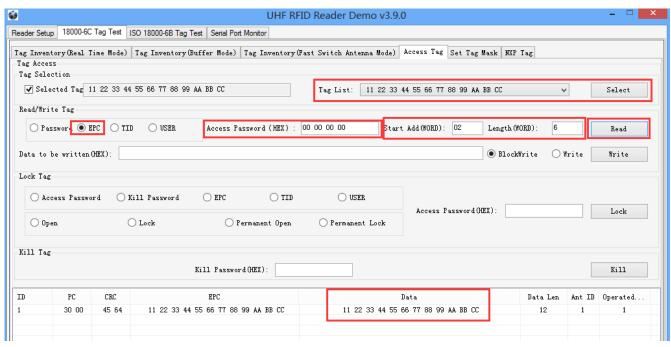
Note that the maximum write length at one time is 32 Words (64 bytes, 512bits).
