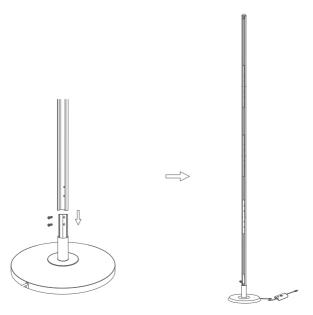
Straighten the silicone strip light. Connect the wires on the silicone strip light to the wires in the lamp base (wires should be connected by color)
