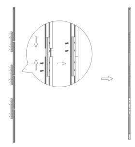
Tips: Before tightening the screws, make sure two poles stay close to each other firmly to avoid large gaps that might cause incline or light leak.
