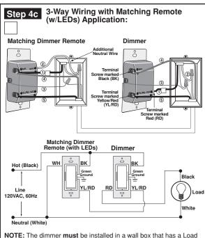
**NOTE:** The dimmer **must** be installed in a wall box that has a Load connection. The matching remote **must** be installed in a wall box with a Line Hot connection and a Neutral connection. A Neutral wire to the matching remote needs to be added as shown. If you are unsure about any part of these instructions, consult a qualified electrician.
