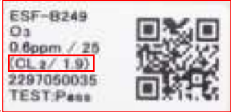
Typical label indicating replacement gas and conversion factor (Example: Replacement gas: Chlorine (Cl 2 ), conversion factor: 1.9)
