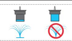
When the Rain Sensor container is full (rainfall of at least 5 mm) it sends the stop signal to the programmers to which it has been associated via the myClaber App.
