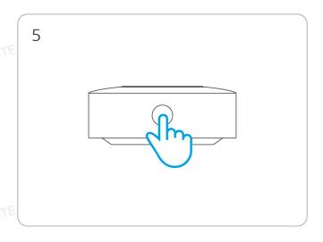
Long press the pairing button for 5 seconds.
