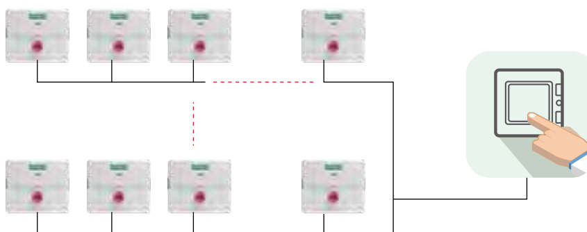
Figure 4.9 Connection diagram of multiple control boxes
