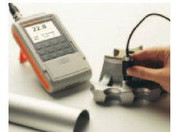
ISOSCOPE® FMP30 using probe FTA3.3H
