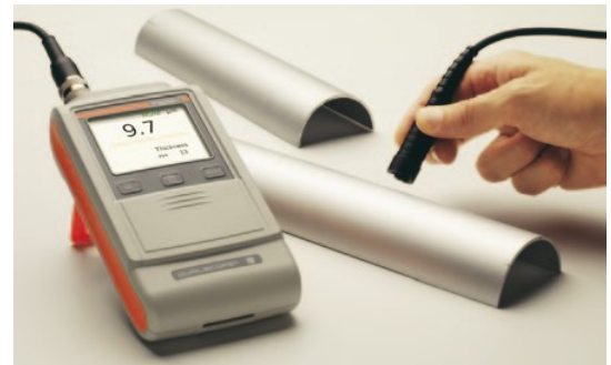
DUALSCOPE® FMP20 using the probe FTD3.3
