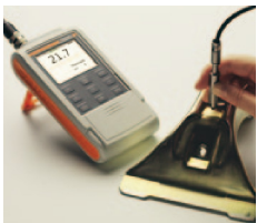
DELTASCOPE® FMP10 using the probe FGAB1.3
