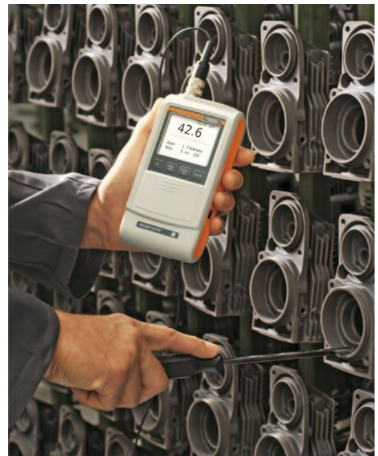
Measurements using the internal probe FAI 3.3-150
