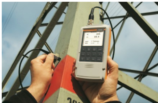
DUALSCOPE® FMP40 using the duplex probe FDX13H
