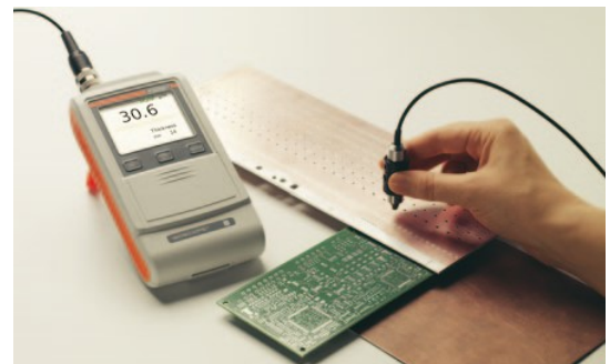
ISOSCOPE® FMP10 using the probe FTA3.3-Cu
