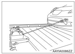
9. Secure the vehicle to the flatbed by using wheel baskets at all 4 wheel positions.
