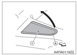
5. Remove the 10mm access cover bolt (A) and turn the 2 plastic clips (B) and remove the cover (1).
