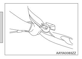
4. Make sure the winch cable remains fully connected to the recovery hook and does not interfere with surrounding area, take up the slack from the cable.
