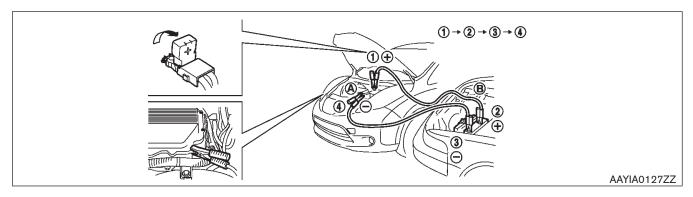
1. If the booster battery is in another vehicle (B), position the two vehicles (A and B) to bring their 12V batteries into close proximity to each other.
