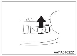
If possible, immobilize the vehicle with the electrically operated parking brake before turning the 12V system OFF and stabilize it with a wheel chock(s). Stabilize the vehicle with wooden blocks or by removing air from the tires.
