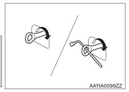
3. Attach the winch cable securely to the recovery hook.
