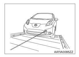
8. Be careful not to pull the vehicle too close to the winch. Doing so will cause excessive downward force being applied to the recovery hook. Too much downward force may result in vehicle damage. Lower the flatbed and finish rolling the vehicle forward if necessary.
