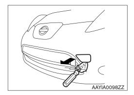
2. Securely install the recovery hook as illustrated. The recovery hook is located in the tool kit area in the left side of the cargo area.
