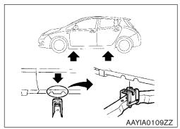
2. Loosen each wheel nut one or two turns by turning it counterclockwise with the wheel nut wrench. Do not remove the wheel nuts until the tire is off the ground.
