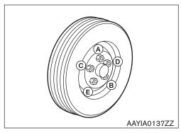
5. Securely torque the wheel nuts in an alternating pattern to 80 ft-lbs (108 Nm).
