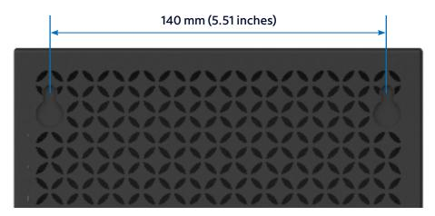
**Note**: The screws should protrude from the wall so you can fit the device between the head of the screws and the wall. If you install the screws in drywall, use hollow wall anchors to ensure the unit does not pull away from the wall due to prolonged strain from the cable and power connectors.
