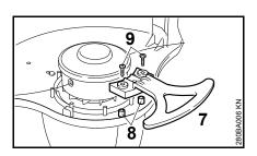
Place the bumper (7) on the pegs (8) and locators in the deflector and secure in position with the two screws (9).
