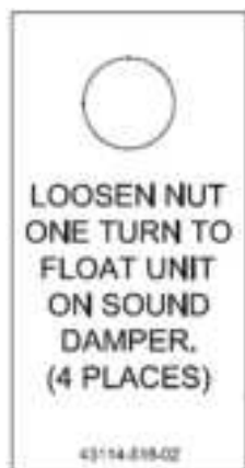
Figure 25 - Loosening the Nut One Full Turn (Four Places) Label
