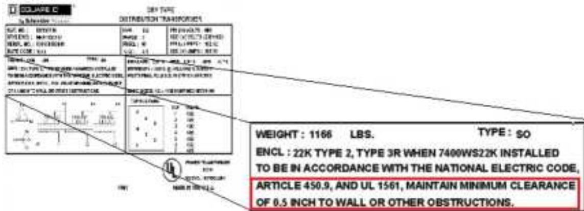
Figure 14 - Minimum Distance Marked on Nameplate NEC 450.9
