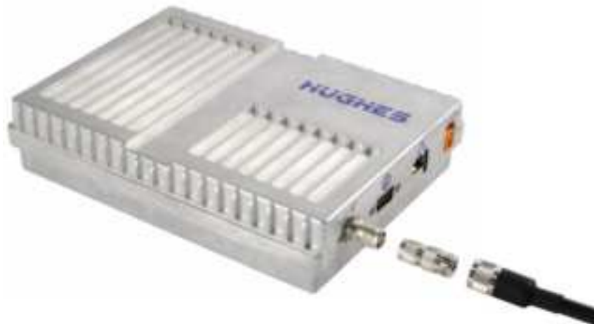
Figure 32: Connect cable to TNC connector on IDU
